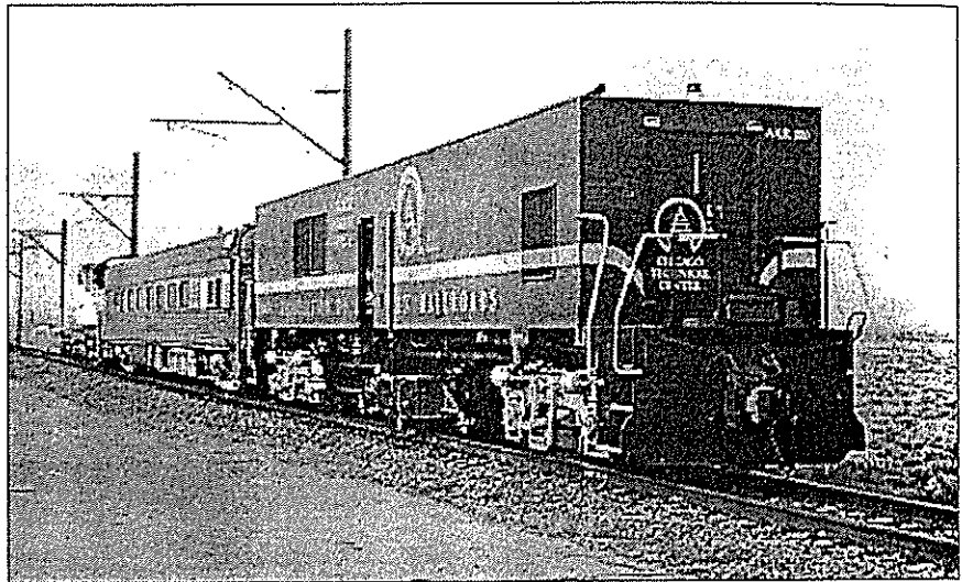
Exhibit 12. Track Loading Vehicle (TLV) Consist at TTC
